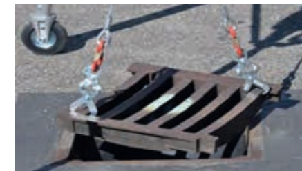
Loosen, lift and drive of manhole covers (max. 500 kg) with winch
