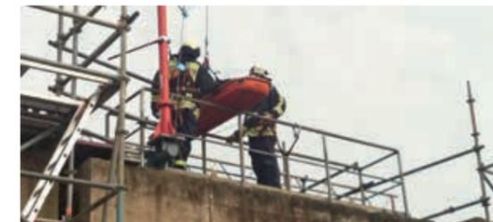
The PHK II-E and the PHK II-S is capable of securing three people combined with HSRG. Secure climbing into and out of tanks, vessels or silos. In case of accident or injury, a person can be rescued safely and quickly by just one person and swing out of the hazard zone.
