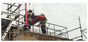
The PHK II-S, the PHK II-E and the PHK II-E XL are capable of securing one person combined with HSRG. Secure climbing into and out of tanks, vessels or silos. In case of accident or injury, the person can be rescued safely and quickly by just one person and swing out of the hazard zone.
